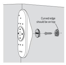
**NOTE**: If you are mounting the Remote Holder onto drywall, use drywall anchors.
